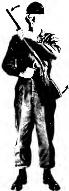
Correct cocking procedure with right hand gripping lever, left hand starts cocking action.
